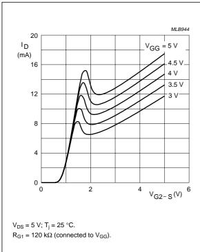
Fig.12 Drain current as a function of gate 2 voltage; typical values; see Fig.18.
